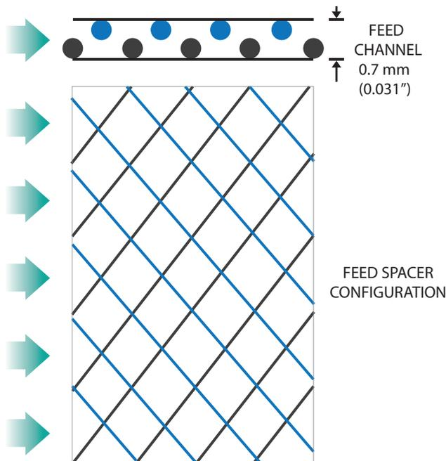
Figure 1. Configuration of a feed channel and a feed spacer net
