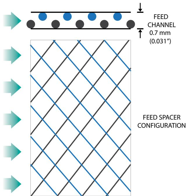
Figure 2. Configuration of a feed channel and a feed spacer net
