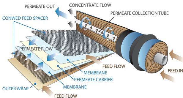
Figure 1. Schematic configuration of spiral wound membrane element
